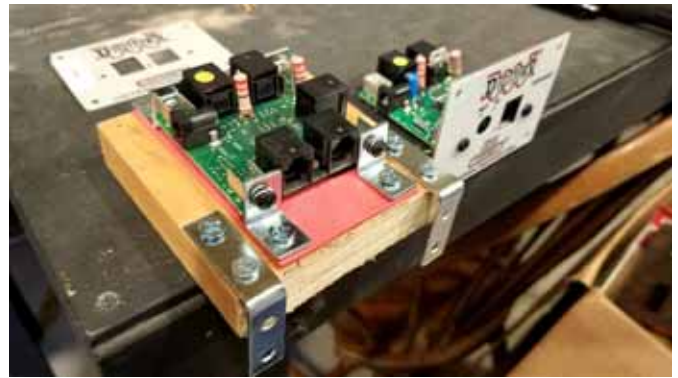
The entire assembly is ready to be mounted onto the module leg.
