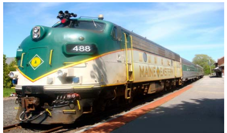
FL-9 built in med-1950's by General Motors Electro-Motive Division for the New Haven Railroad.
