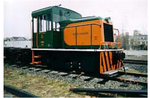
General Electric 70-ton diesel-electric as rehabilitated by the Providence & Worcester Railfan Club, Inc in New Haven Colors, Nov 25, 2004
