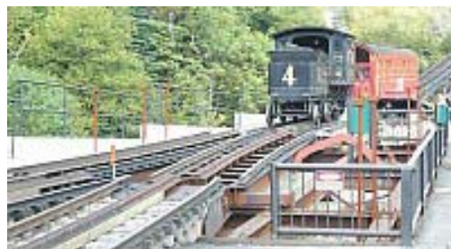
Picture above shows the new hydraulic switch being thrown. Below it is all set for the train to pass through. These pictures were taken at Marshfield Base.
