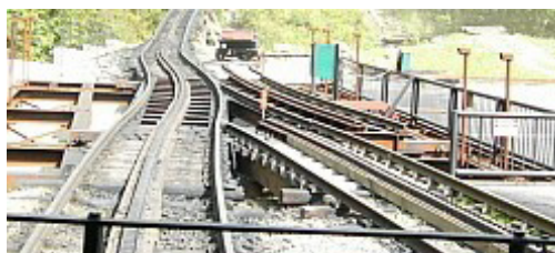
Picture above shows the new hydraulic switch being thrown. Below it is all set for the train to pass through. These pictures were taken at Marshfield Base.
