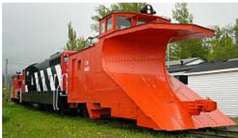
Push Plow 3460 one of many plows used to clear the snow sometime higher than the train.
